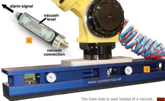
The blue-colored EOAT shown in Fig 5 is a self-contained vacuum lifting head. This head incorporates all the items needed to provide the user a vacuum-gripping device. This particular unit utilizes vacuum "foam" instead of traditional vacuum cups. This vacuum foam is shown in greater detail in Fig 6.
