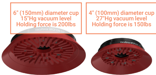
Figure 5: Examples of vacuum cup lifting forces.
