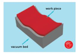
vacuum being achieved is only 3"Hg (due to leakage through the MDF), the holding force will be reduced by 90%, which equates to 6.4N. This might be enough for a machining process, such as simple hole drilling, but if there is a large side load during profile machining, the vacuum level may need to be higher. This is when the open MDF sheet should be covered by a plastic sheet.
