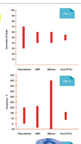
sense that a vacuum cup has fallen into the food packaging that typically contains baked goods like bread loaves, rolls, and buns. The wear resistance of silicone compared to NBR is poor. Typically on an abrasive surface such as cardboard, an NBR cup would last at least twice as long. That said, silicone has a better seal on the cardboard, and consequentially, a higher vacuum level can be achieved, which offers higher load capacity for the tool. One feature trades off against the other.
