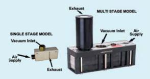
right image. The difference between a single-stage and multistage venturi, in practical terms, is that the multi units use less compressed air to generate vacuum flow and, because of this, typically are used in larger vacuum-flow applications. Benefits and comparisons between the multistage and single-stage venturi are discussed in the September/October 2008 issue ("The Vacuum Venturi Explained").
